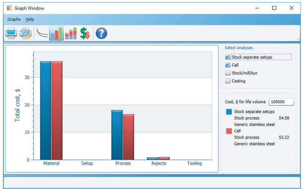
4. The total cost per part for the part produced in a cell is \$53.22 compared with \$54.58 for the part produced on separate setups. However, the cost of material is \$35.77 and therefore the non-material cost savings from machining in the cell is just under 9% (\$17.45 compared with \$18.81).
